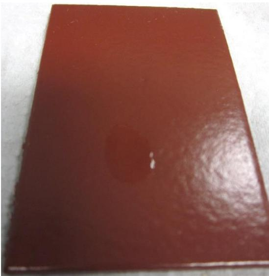
Fig. 2.1 Drop totally spread. Surface tension of the coating is higher than the liquid.
