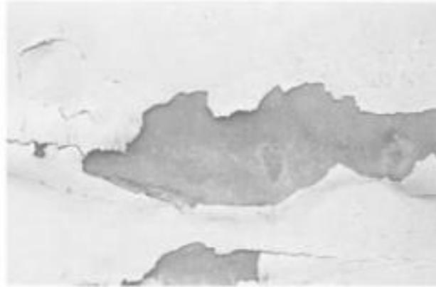
**Fig. 1.2 Detachment of a coating from oil-contaminated substrate.**
