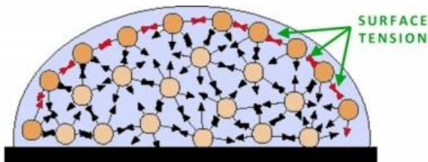
**Fig. 1.1 Enhancement of the intermolecular attractive forces at the surface is called surface tension.**
