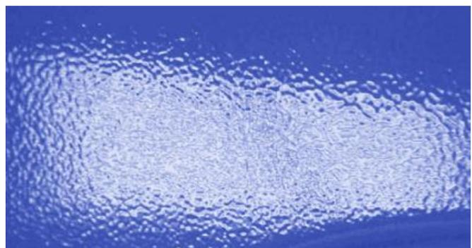
**Fig. 1.3 Orange peel defect.**
