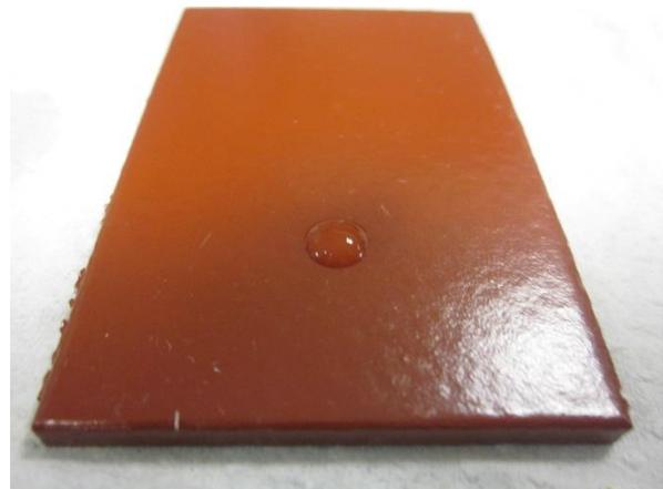
Fig. 2.2 Drop-like shape. Surface tension of the coating is lower than the liquid.
